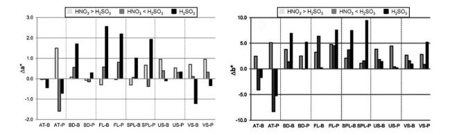
**Figure 2.** Variations in colour parameters "a" and "b" (in L.a.b. colour space) after each ageing test for the "*bush hammered finish*, (B)" and the "*polished finish*, (P)" natural stones. (Test samples were codified as; AT: Albox travertine, BD: Boñar dolostone, FL: Fraga limestone, SPL: Santa Pudia limestone, US: Uncastillo sandstone, VS: Villaviciosa sandstone), (Vazquez, et al., 2016).
