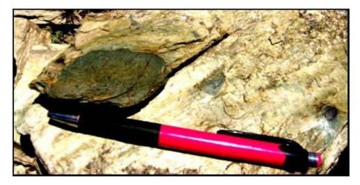
**Figure 2**. Rock fragments with variable size within phyllite of Bagrıkurt Formations (pen:13 cm in length).
