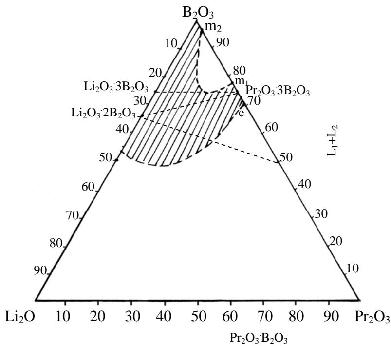
**Figure 1.** Diagram of glass formation in triple system  $\text{Li}_2\text{O}-\text{Pr}_2\text{O}_3-\text{B}_2\text{O}_3$ .
